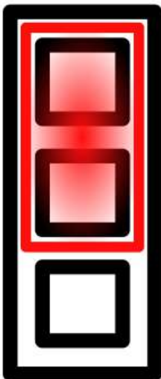
CAN Termination ON
