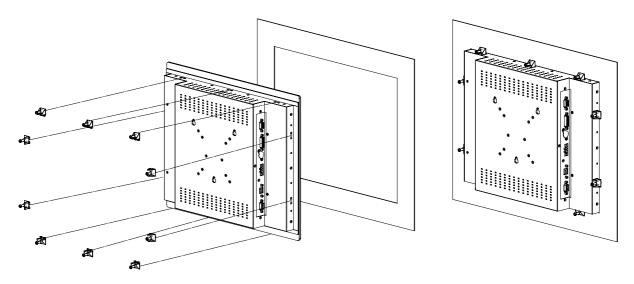
Figure 2.2 Panel Mounting (392 x 292 mm)
