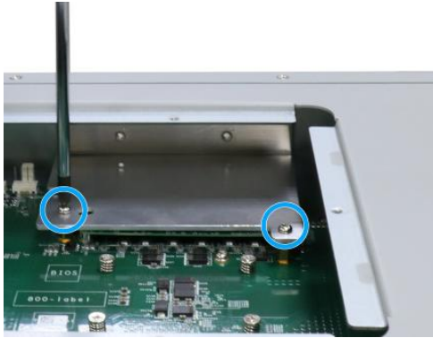
Screws on top of the heat spreader
