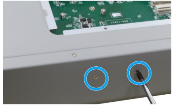
Screws at the back of the enclosure
