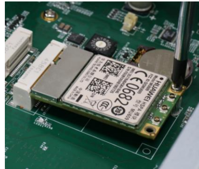
Secure the module with a screw
