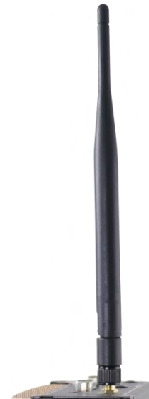
Attach external antenna
