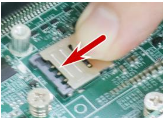
Push the SIM holder in the direction shown
