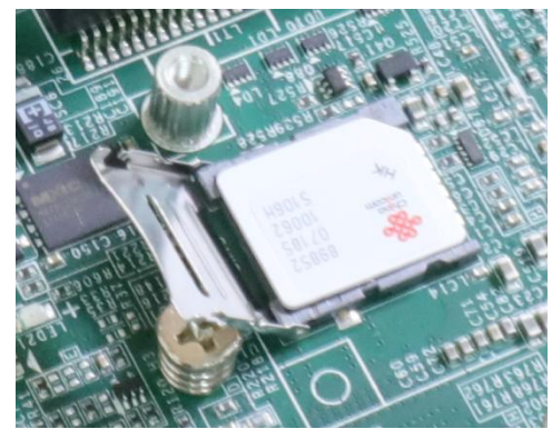
Flip open the holder and place SIM
