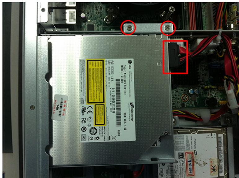
5. Connect the DVD ROM to 4-pin power connector using the power adapter provided in the accessory box.
