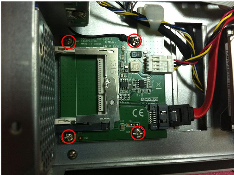
2. Plug the power cable into the CFAST module and connect the other end to the 4-pin power connector.
