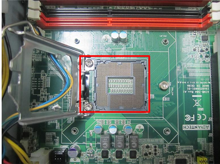
4. Install the CP, taking note of the direction of the notched corner.
