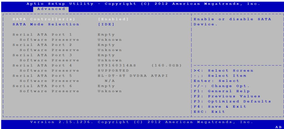
Users can also set the HDD mode to either IDE, AHCI, or RAID.
