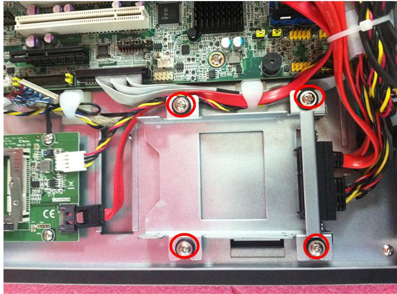
2. Insert the HDD and tighten the affixing screws (provided in the accessory box).
