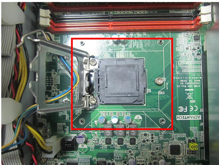
3. Remove the CPU pin cap.
