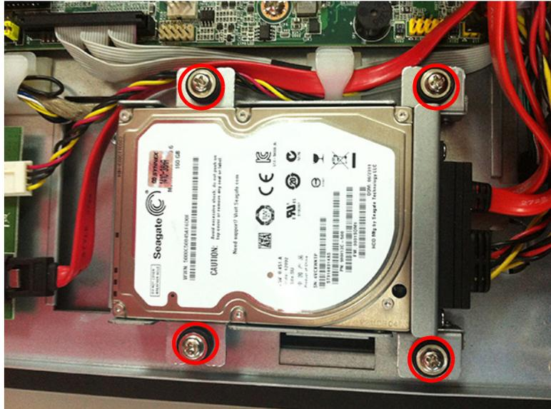
**Note!** *If installing two HDDs, insert them together and fasten the screws on the HDD bracket. The thickness of the HDD must not exceed 9.5 mm (0.37 in). Otherwise, only one HDD or SSD will be able to be installed.*
