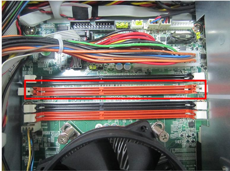
3. Insert the memory and then return the lever to its original position.
