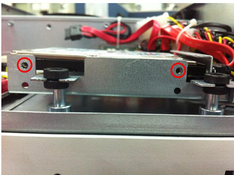
3. Replace and fasten the four screws to secure the HDD bracket in place.
