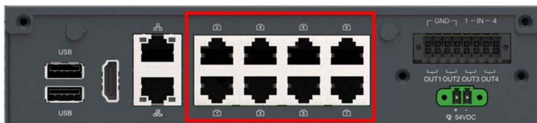
Figure 2.6 Power over Ethernet (PoE)
