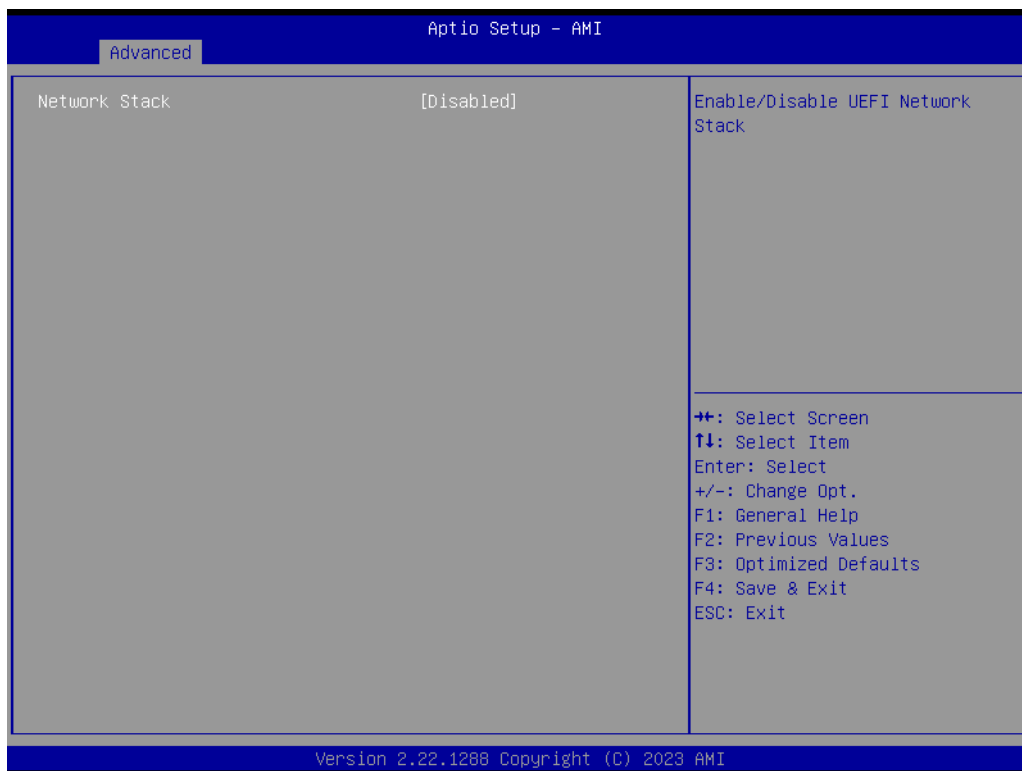
Figure 3.33 Network Stack Configuration
