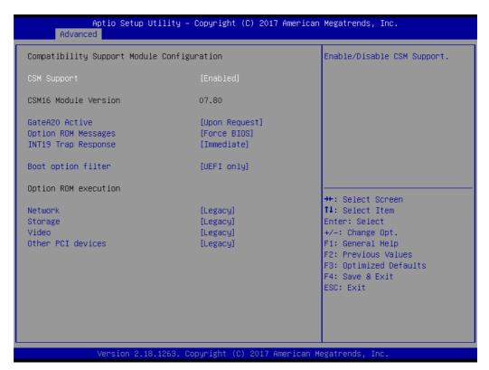
Figure 3.28 CSM Configuration
