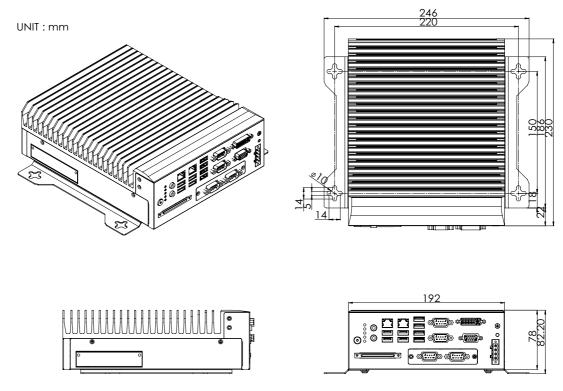
Figure 1.1 MIC-7700 Mechanical Dimension Drawing
