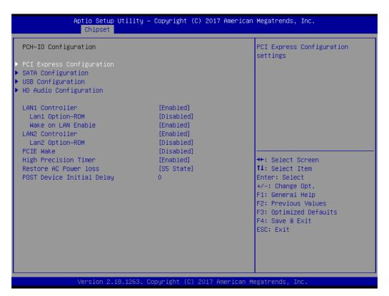
Figure 3.37 PCH-IO Configuration
