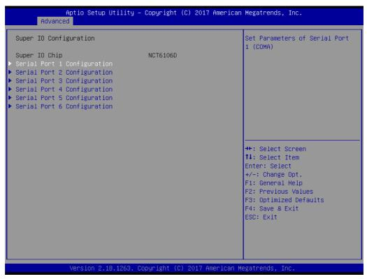
Figure 3.16 Super IO Configuration
