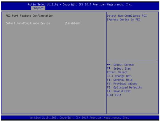
Figure 3.35 PEG Port Feature Configuration
