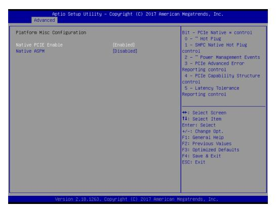
Figure 3.4 Platform Misc Configuration
