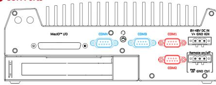
The system provides four COM ports to communicate with external devices. The COM ports are implemented using industrial-grade ITE8786 Super IO chip (-40 to 85°C) and provide up to 115200 bps baud rate. COM1 and COM2 (in red) are software-configurable RS-232/422/485 ports. COM3 and COM4 (in blue) are standard 9-wire RS-232 ports. The operation mode of COM1 and COM2 can be set in BIOS setup utility. The following table describes the pin definition of COM ports.
