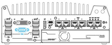
VGA connector is the most common video display connection. The VGA output supports up to 1920x1200@60Hz resolution. The system supports triple independent display outputs by connecting display devices to VGA, DVI and DisplayPort connection. To support multiple display outputs and achieve best VGA output resolution in Windows, you need to install corresponding graphics drivers.
