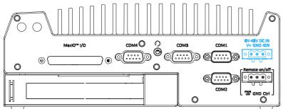
The system accepts a wide range of DC power input from 8 to 48V via a 3-pin pluggable terminal block, which is fit for field usage where DC power is usually provided. The screw clamping mechanism on the terminal block offers connection reliability when wiring DC power.
