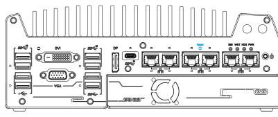
The reset button is used to manually reset the system in case of system halt or malfunction. To avoid unexpected reset, the button is purposely placed behind the panel. To reset, please use a pin-like object (eg. tip of a pen) to access the reset button.
