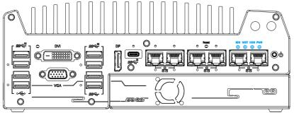
There are four LED indicators on the I/O panel: IGN, WDT, HDD and PWR. The descriptions of these four LED are listed in the following table.
