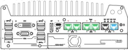
The ports marked in green/ black are Power over Ethernet (PoE) ports implemented with Intel I225-IT 2.5G Ethernet controller, and marked in blue is implemented using Intel® I219-LM controller that supports Wake-on-LAN and is also compatible with Intel® AMT (Active Management Technology) to support advanced features such as remote SOL desktop and remote on/ off control. The four PoE+ ports feature panel screw fix holes (indicated in red) for a firm and secure connection.
