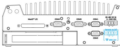
The "Remote On/ Off" 3-pin connection allows for the connection of an external non-latched switch to turn on/ off the system. It is useful when the system is placed in a cabinet or a not easily accessed location. You may connect an external status LED (20mA) indicator by connecting to PWR LED and GND.
