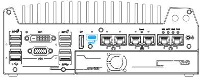
The system's USB 3.2 Gen2x2 type-C port offers up to 20Gbps of data transfer bandwidth, and is implemented via the native xHCI (eXtensible Host Controller Interface) controller. The port is backward compatible with USB3.2 Gen.1 USB 2.0, USB 1.1 and USB 1.0 devices via a USB hub (not included) to connect to external devices.
