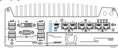
The system has a DisplayPort (DP) output which is a digital display interface that mainly connect video source and carry audio to a display device. When connected to a DP, it can deliver up to 8K UHD (7680 x 4320 @ 60Hz) in resolution. The system is designed to support passive DP adapter/ cable. You can connect to other display devices using DP-to-HDMI cable or DP-to-DVI cable.
