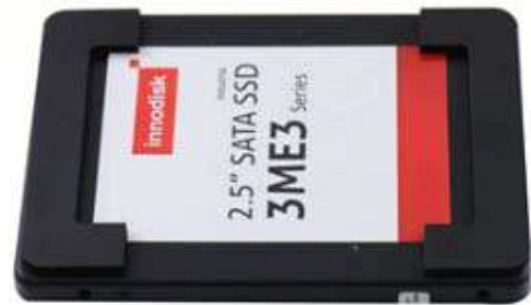
Attach PORON if you are installing a 7mm HDD/ SSD
