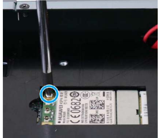
Secure the card with a screw
