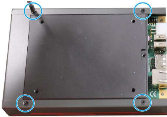
Screws holding the flattop heatsink with enclosure
