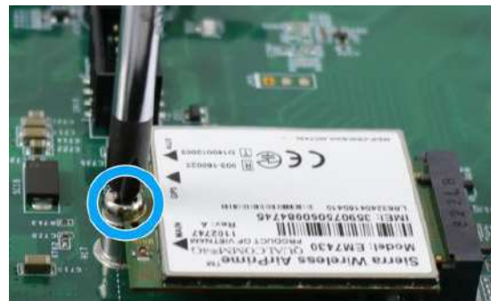
Secure with a M3 P-head screw
