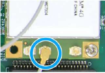
Clip on IPEX-to-SMA cable
