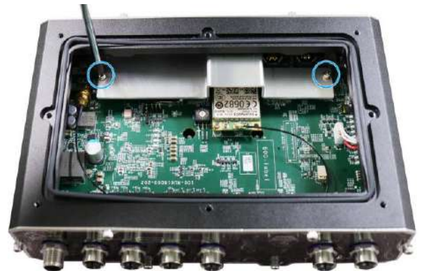
Secure with screws indicated
