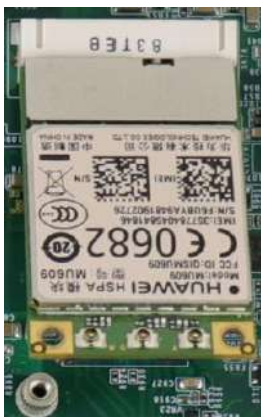
Insert at 45 degree angle
