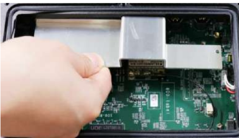
Place heatsink back on the modules
