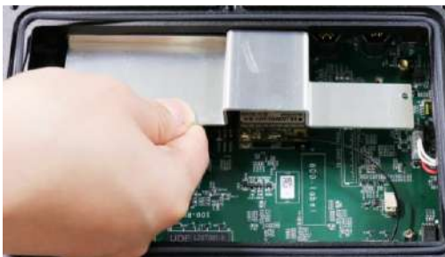
Place heatsink back on the modules
