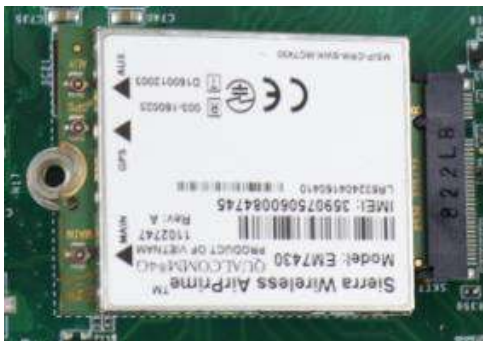
Insert on a 45° angle
