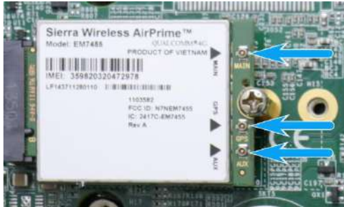
Clip on the IPEX-to-SMA cable
