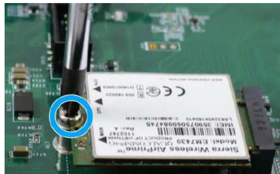
Secure with a M2.5 P-head screw
