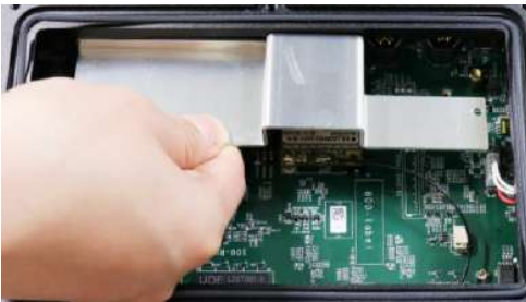
Place heatsink back on the modules
