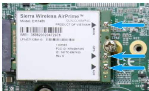
Clip on the IPEX-to-SMA cable
