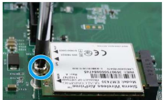
Secure with a M2.5 P-head screw
