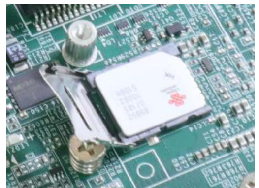
Flip open the holder and place SIM
