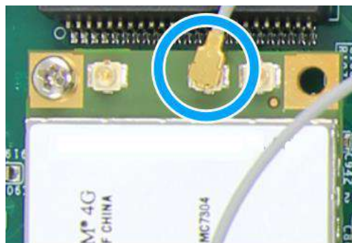
Clip on the IPEX-to-SMA cable
