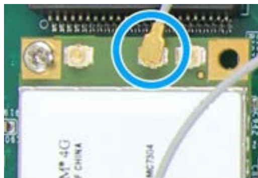
Clip on the IPEX-to-SMA cable
