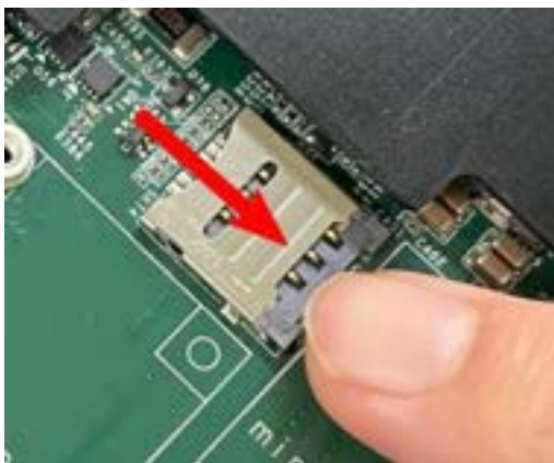
Push the SIM holder in the direction shown
