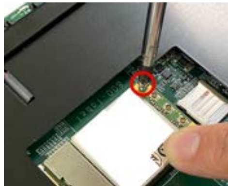
Secure the card with a screw
