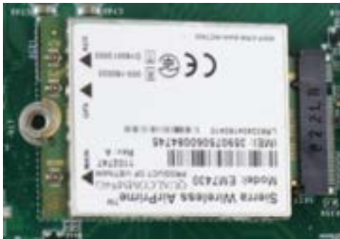
Insert on a 45° angle
