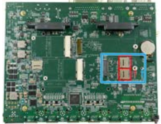
Location of M.2 B key and internal SIM card slot (heat spreader removed)
