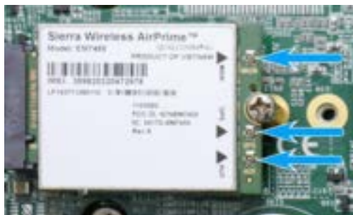
Clip on the IPEX-to-SMA cable
