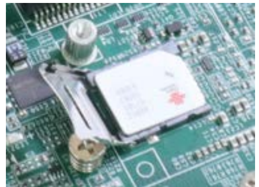
Flip open the holder and place SIM
