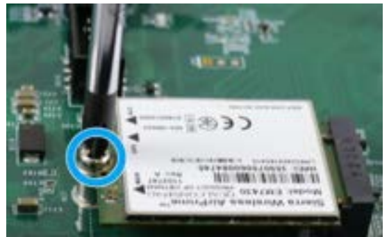
Secure with a M2.5 P-head screw
