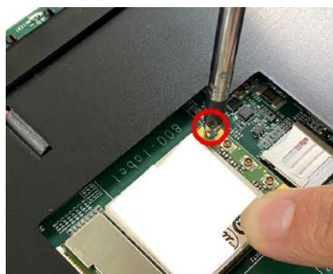
Secure the card with a screw
