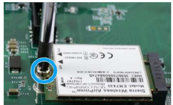
Secure with a M2.5 P-head screw
