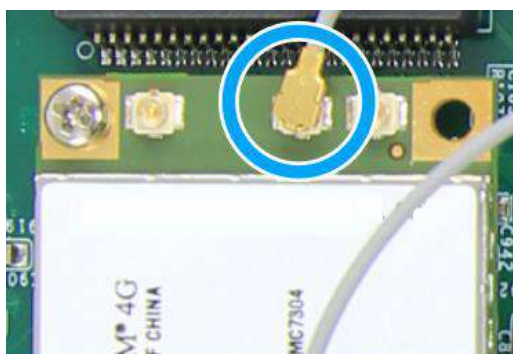
Clip on the IPEX-to-SMA cable
