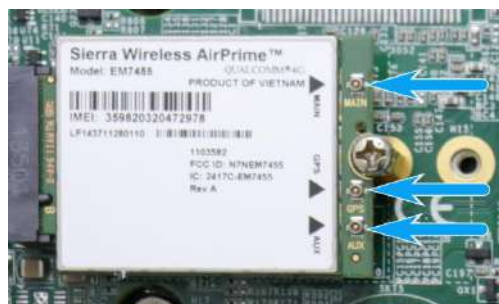
Clip on the IPEX-to-SMA cable
