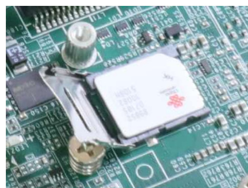
Flip open the holder and place SIM
