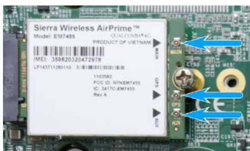
Clip on the IPEX-to-SMA cable
