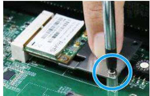
Secure the card with a screw
