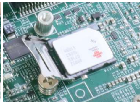
Flip open the holder and place SIM
