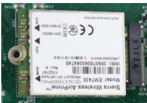
Insert on a 45° angle
