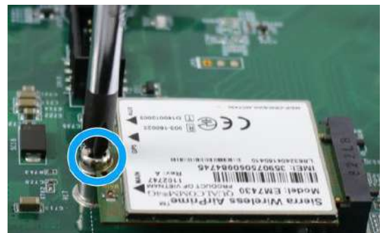
Secure with a M2.5 P-head screw
