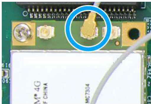
Clip on the IPEX-to-SMA cable
