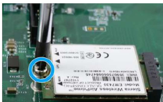
Secure with a M2.5 P-head screw
