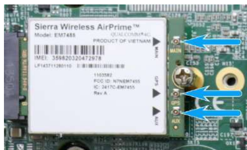
Clip on the IPEX-to-SMA cable
