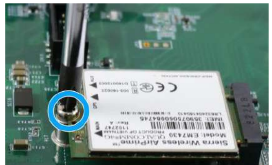
Secure with a M2.5 P-head screw
