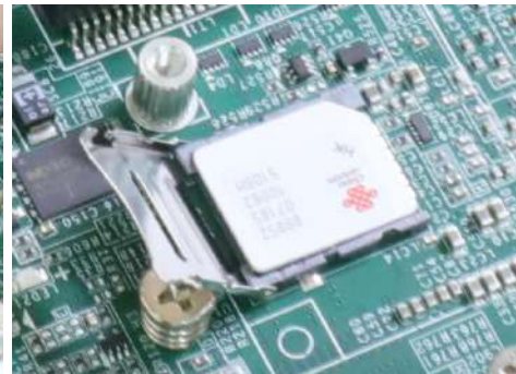
Flip open the holder and place SIM
