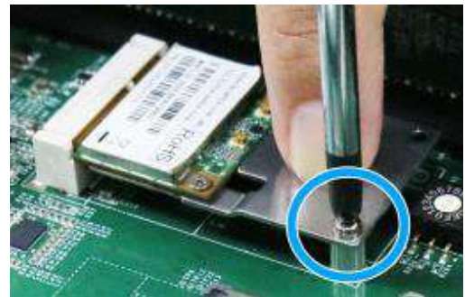
Secure the card with a screw
