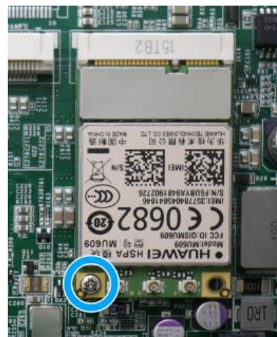
Secure the card with a screw
