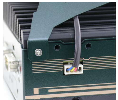
Plug in the 4-pin power connector
