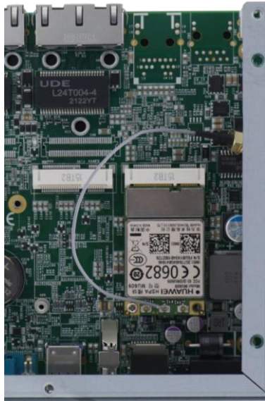
Clip on the IPEX-to-SMA cable
