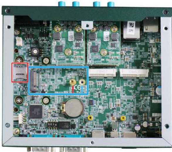
M.2 B key and internal SIM card slot
