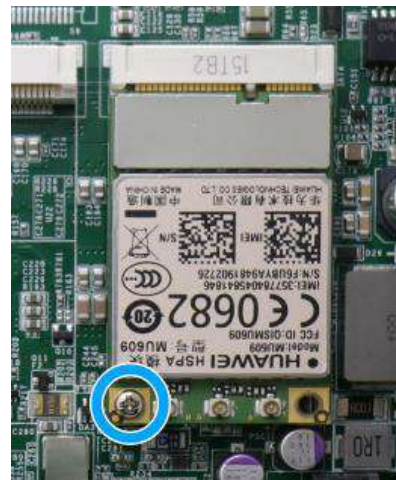
Secure the card with a screw
