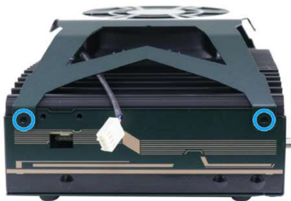
Secure the two screws
