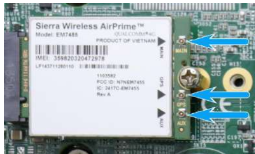
Clip on the IPEX-to-SMA cable
