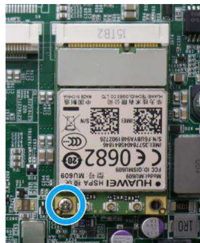
Secure the card with a screw
