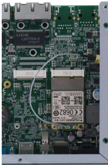
Clip on the IPEX-to-SMA cable
