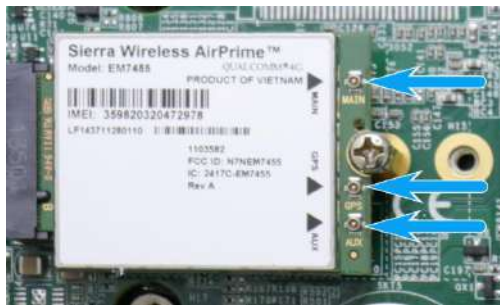
Clip on the IPEX-to-SMA cable
