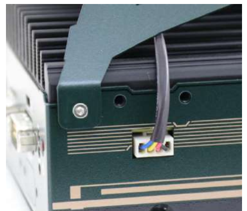
Plug in the 4-pin power connector
