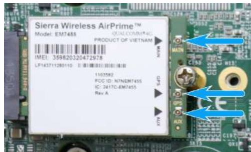
Clip on the IPEX-to-SMA cable
