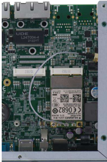
Clip on the IPEX-to-SMA cable
