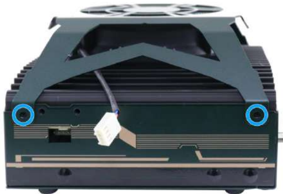
Secure the two screws
