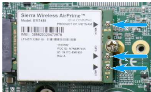
Clip on the IPEX-to-SMA cable
