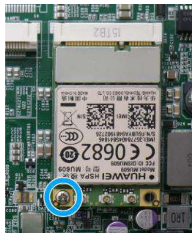
Secure the card with a screw
