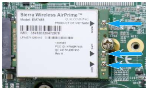
Clip on the IPEX-to-SMA cable
