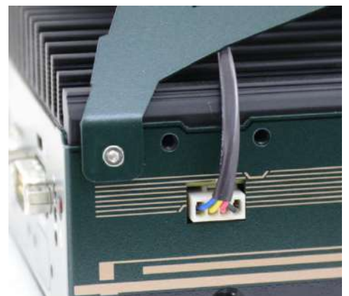
Plug in the 4-pin power connector
