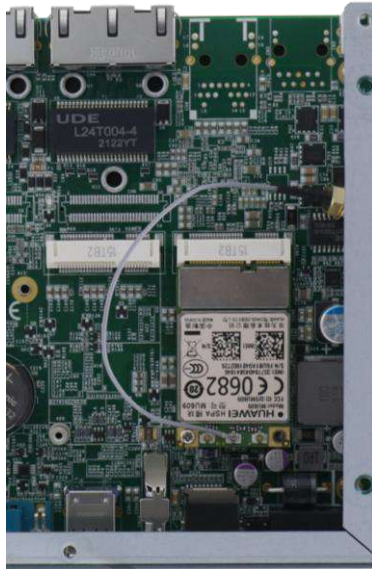
Clip on the IPEX-to-SMA cable
