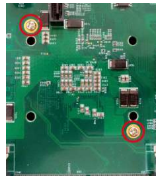
Secure two M3 P-head screws on the opposite side
