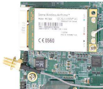
Clip on IPEX-to-SMA cable
