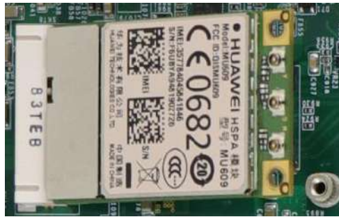
Insert on 45 degree angle
