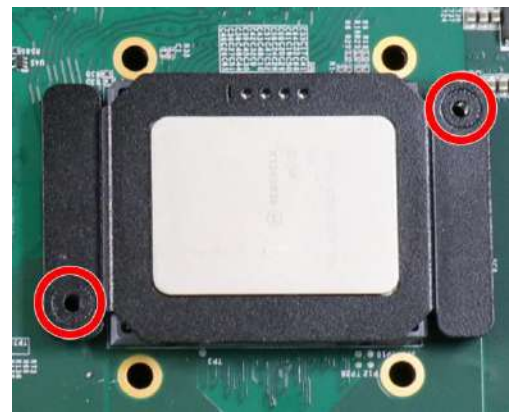
Place the CPU retention bracket on while matching the screw holes
