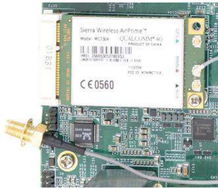
Clip on IPEX-to-SMA cable
