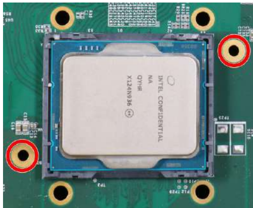
Screw holes for CPU retention bracket
