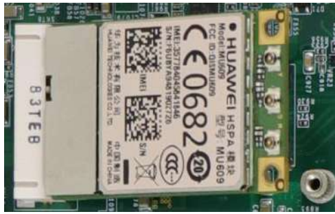
Insert on 45 degree angle
