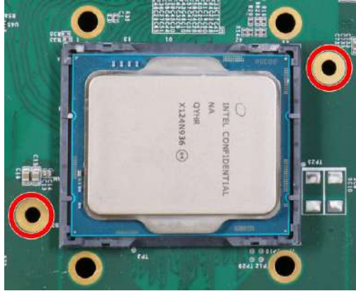
Screw holes for CPU retention bracket
