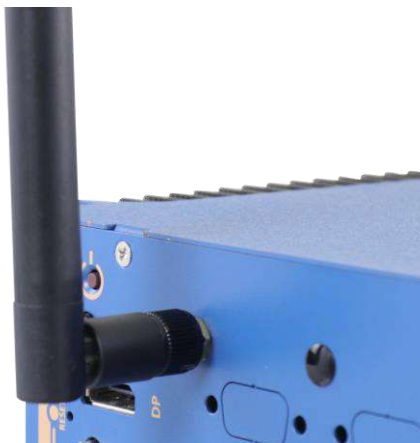
Clip on IPEX-to-SMA cable
