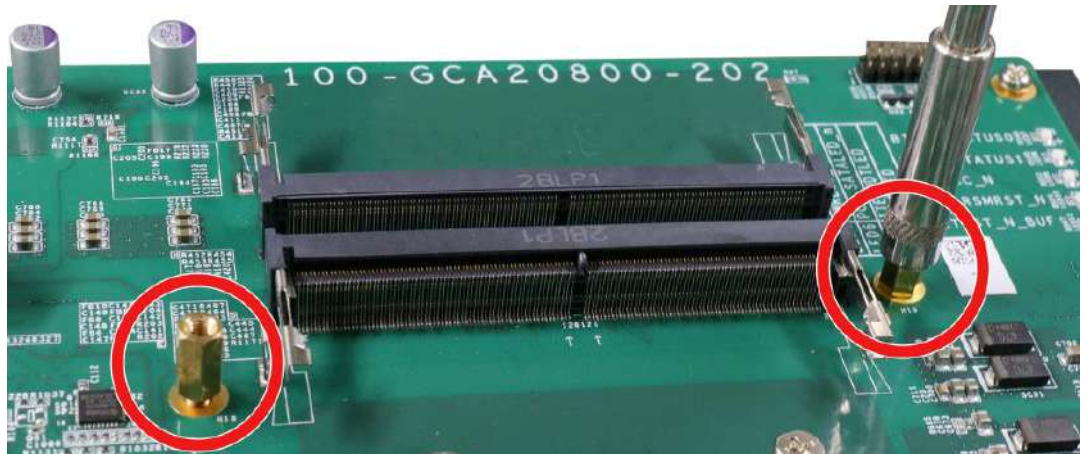
Remove the copper stands supporting the memory module's heatsink
