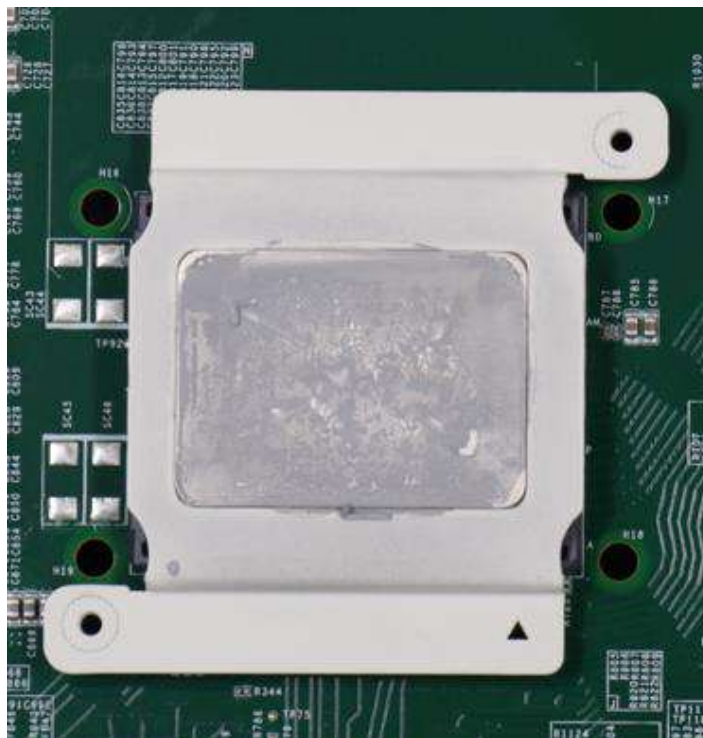
CPU retention bracket (holder)
