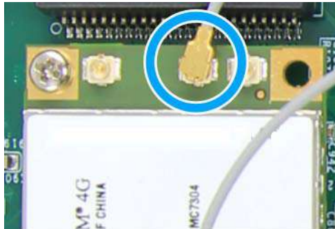
Clip on IPEX-to-SMA cable
