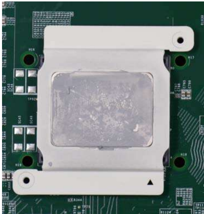
CPU retention bracket (holder)
