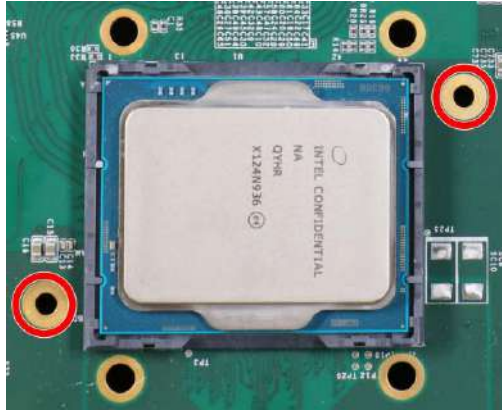
Screw holes for CPU retention bracket
