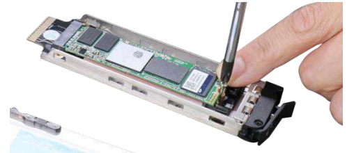
Secure with a screw
