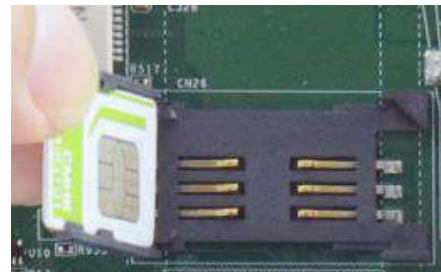
Insert SIM card with pins facing up
