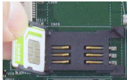
Insert SIM card with pins facing up
