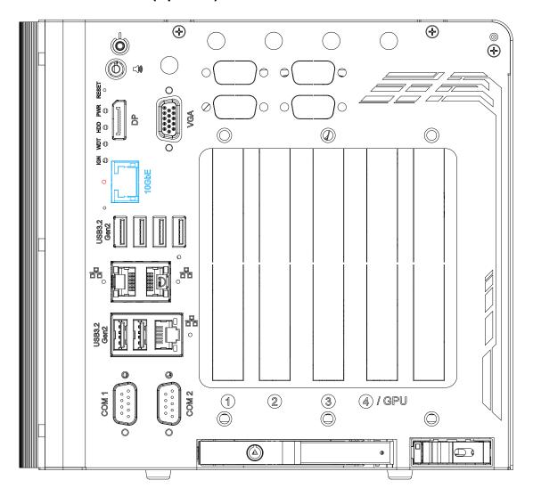
The optional high-speed data transmission 10G Ethernet port is backward compatible with 5GBASE-T and 2.5GBASE-T to work with NBASE-T industrial cameras. Indicated in **red** is a screw-lock hole for the corresponding Ethernet port.
