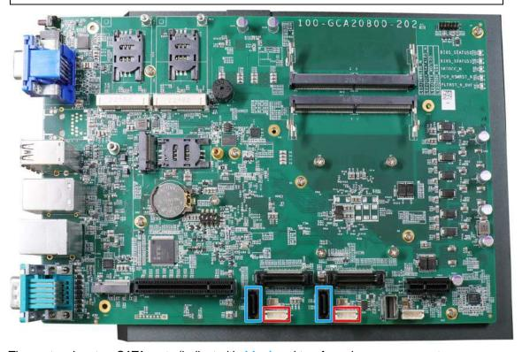
The system has two SATA ports (indicated in **blue**) and two four pin power connectors (indicated in **red**). Only one of the SATA and power connector will be connected to the front-accessible tray, so users only need to install the HDD/ SSD to the easy-swap tray. Please refer to the following instructions on how to install a 2.5" SATA HDD/SSD.
