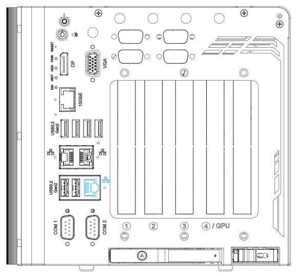
The system has a GbE ports on its I/O panel and support Wake-on-LAN functions. The GbE port is implemented with Intel® I219-LM controller with one dedicated PCI Express link for maximum performance. When the Ethernet connection is established, the LED indicators on the RJ45 connector represents the following connection statuses:
