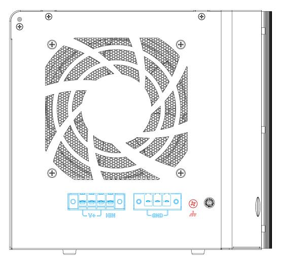
The system accepts a wide range of DC power input from 8 to 48V via a 4-pin and 3-pin pluggable terminal block, which is fit for field usage where DC power is provided. The screw clamping mechanism on the terminal block offers connection reliability when wiring DC power. In addition to DC power input, this terminal block can also accept ignition signal input (IGN) with a grounding point (indicated in **red**) for in-vehicle applications.
