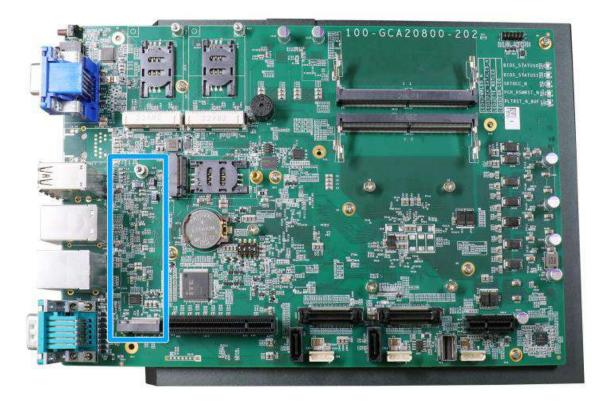
The system has a Gen4x4 PCIe M.2 2280 slot for you to install an NVMe SSD for the ultimate performance. The NVMe SSD offers noticeable performance advantages over 2.5" SSDs for smoother operating system operation and responses.
