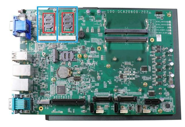
The system provides two mini-PCle sockets (indicated in blue) that is in compliance with mini-PCle specification rev. 1.2. The mini-PCle sockets are designed with a SIM card (slot indicated in red) support. With a SIM card installed, your system can access the internet via your network provider's 4G/3G network.
