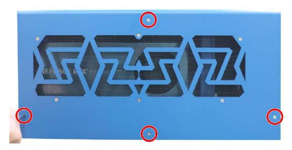
7. Secure the screws indicated on the top of the enclosure.
