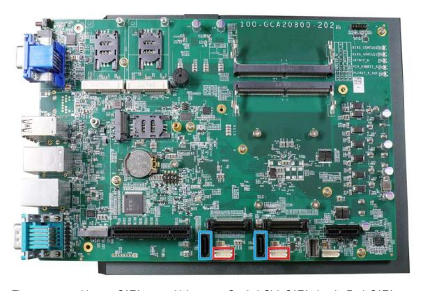
The system provides two SATA ports which support Gen3, 6 Gb/s SATA signals. Each SATA port (indicated in blue) features a 7-pin SATA connector and a 4-pin power connector.
