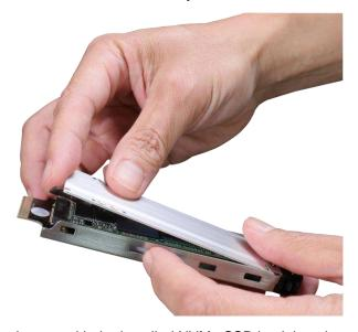
6. Insert the tray with the installed NVMe SSD back into the enclosure, and push the lever back in to complete the installation. The tray is also lockable with the provided key when you purchase this optional kit.
