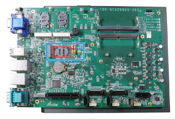
The system has an M.2 2242/ 3052 slot (indicated in **blue rectangle**) with a 5G/ 4G SIM slot (indicated in **red rectangle**). A copper standoff is provided for you to secure onto the motherboard into the **red arrow** location for an M.2 2242 module, or into the **blue arrow** location for an M.2 3052 module. By installing a 5G or 4G M.2 module and SIM card, you can access the internet via the provider's network.
