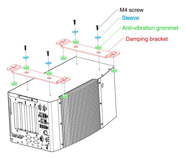
2. Place the system on top of a flat horizontal surface and secure it with screws.
