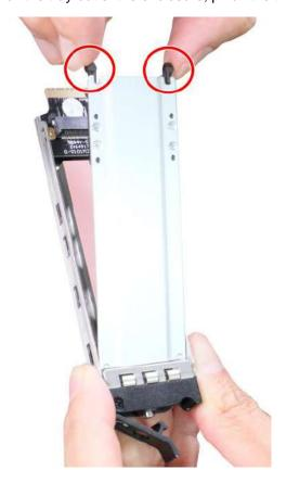
3. Insert the NVMe SSD module on a 45° angle and secure with a screw.
