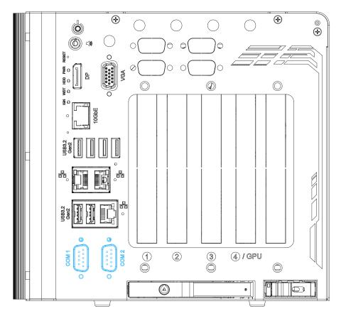
The two COM ports are implemented using industrial-grade ITE8786 Super IO chip (-40 to 85°C) and provide up to 115200 bps baud rate. COM1 and COM2 (in **red**) are software-configurable RS-232/422/485 ports. COM3 and COM4 (in **blue**) are standard 9-wire RS-232 ports. The operation mode of COM1 and COM2 can be set in BIOS setup utility. The following table describes the pin definition of COM ports.
