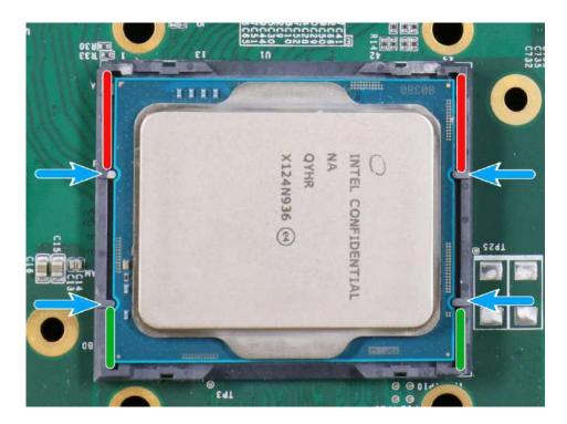
Locate the CPU retention bracket (holder) from the accessory box. Place the retention bracket on the CPU and hold it in place. Make sure the screw holes match the CPU retention bracket's screw holes (indicated by red circles).
