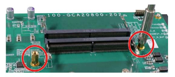
Remove the copper stands supporting the memory module's heatsink
