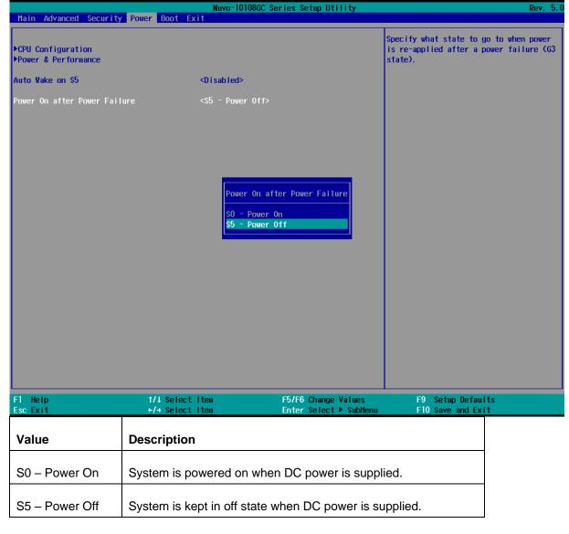
To set "Power On after Power Failure" option:
