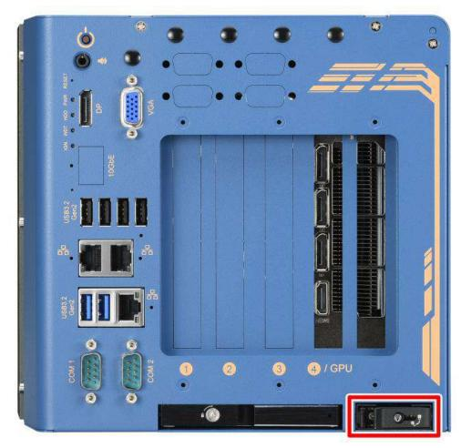
1. Lift the lever in the direction indicated to access the tray.
