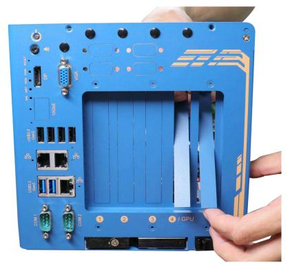
4. Take out the graphics card dedicated bracket and cable and attach the cable sorting peg.
