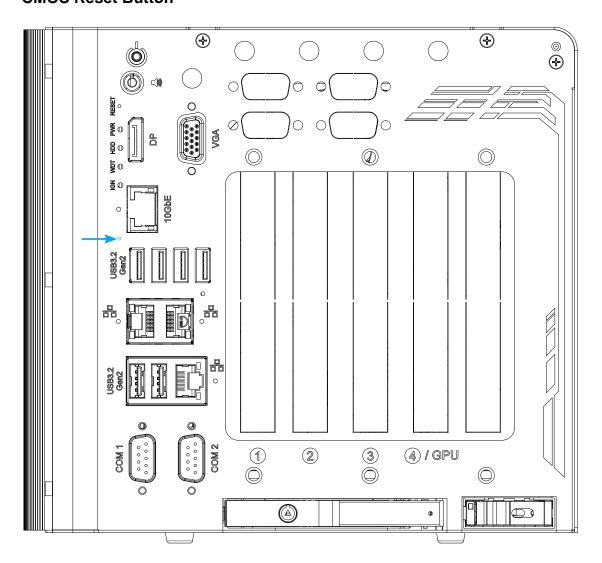
Positioned between 10GbE and USB ports, indicated by the **blue arrow**, the CMOS Reset button is used to manually reset the motherboard BIOS in case of system halt or malfunction. To avoid unexpected operation, it is purposely placed behind the panel. To reset, please use the tip of a pen, press and hold for at least 5 seconds to reset the BIOS.
