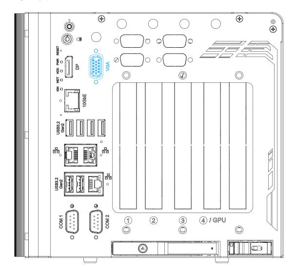
The VGA port is the most common video display connection. The VGA output supports up to 1920x1200@60Hz resolution.
