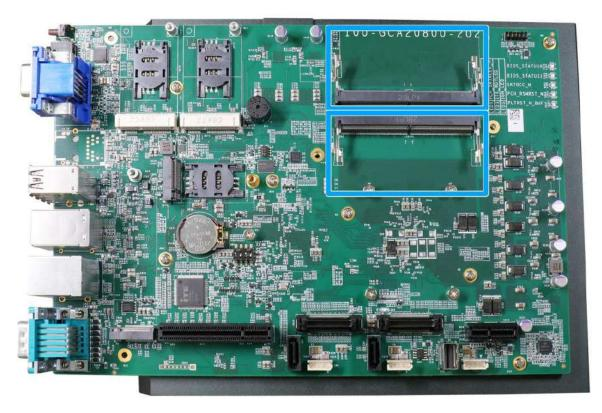
The system motherboard supports two ECC/ non-ECC SODIMM sockets for installing DDR5 memory module up to 64GB. Each slot supports single module DDR5 4800MHz SODIMM up to 32GB capacity.
