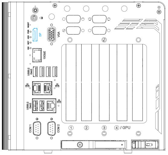
The DisplayPort (DP) output is a digital display interface that mainly connect video source and carry audio to a display device. When connecting a DP, it can deliver up to 4K UHD (4096 x 2304) in resolution. The system is designed to support passive DP adapter/ cable. You can connect to other display devices using DP-to-HDMI cable or DP-to-DVI cable.
