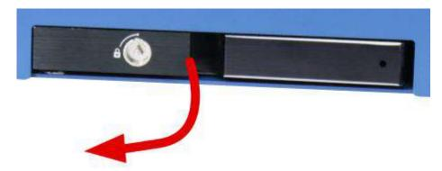
Insert the HDD/ SSD (with labels facing up) and the SATA connector end towards the slot, insert it 3/4 of way in and use the lever to fully push the HDD/ SSD into the slot. You should hear a click sound to ensure the HDD/ SSD is properly inserted and engaged.
