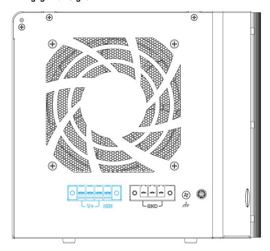
To have ignition power control for in-vehicle usage, you need to supply IGN signal to the system. The IGN input is located on the 4-pin pluggable terminal block (shared with DC power input). Below is the typical wiring configuration for in-vehicle applications.
