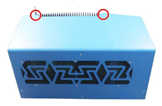
4. On the rear exhaust fan panel, remove two screws indicated in **blue**, and remove four screws indicated in **red** holding the exhaust fan in place.
