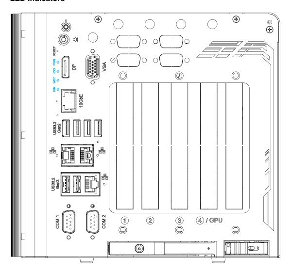
There are four LED indicators on the I/O panel: IGN, WDT, HDD and PWR. The descriptions of these four LED are listed in the following table.
