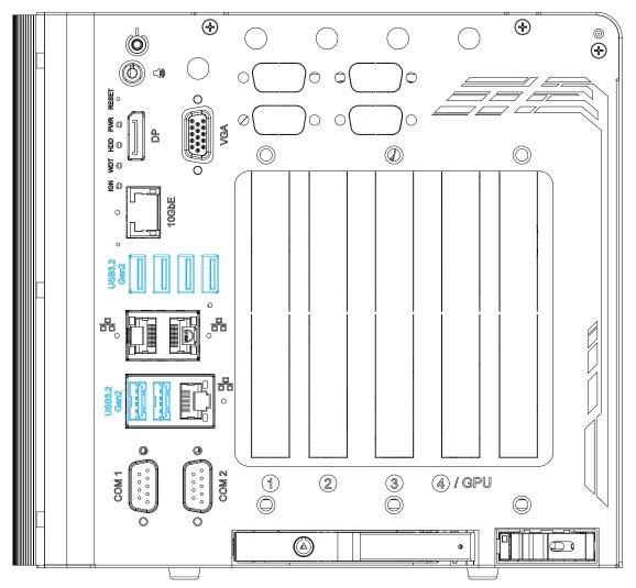
The system's USB 3.1 Gen 2 ports (10Gbps) are implemented via native xHCl (eXtensible Host Controller Interface) controller and are backward compatible with USB3.1 Gen.1 USB 2.0, USB 1.1 and USB 1.0 devices. Legacy USB is also supported so you can use USB keyboard/mouse in DOS environment.
