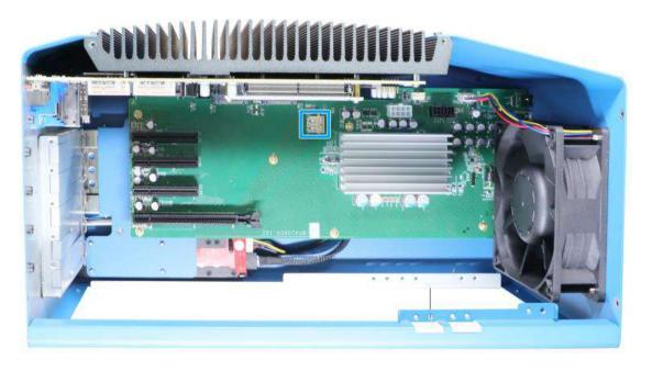
The system's daughter board has an internal USB2.0 port on the PCBA. You can utilize this USB port to connect a USB protection dongle inside the chassis of the system.
