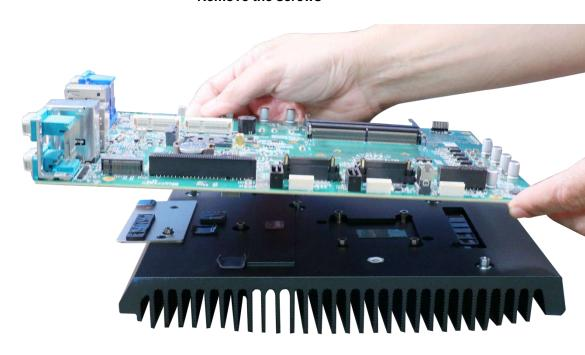
Separate the motherboard from the heatsink
