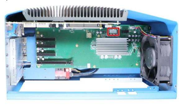
The 8-pin power connector (indicated in **red**) is designed only to support power-consuming PCIe cards, such as frame grabber cards with PoE+. The power budget of the 8-pin connector is limited to 150W, which is insufficient for most modern GPU cards.
