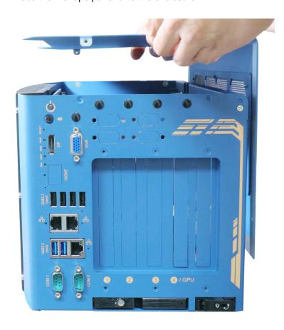
Place L-shape side panel onto the enclosure
