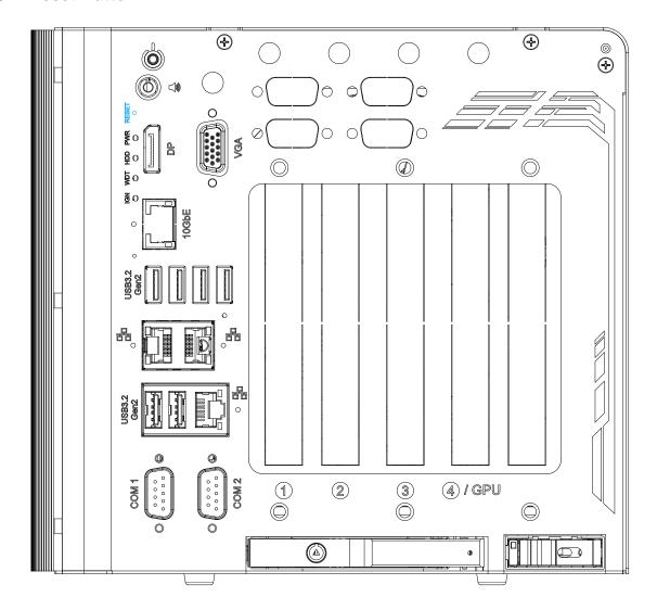
The reset button is used to manually reset the system in case of system halt or malfunction. To avoid unexpected reset, the button is purposely placed behind the panel. To reset, please use a pin-like object (eg. tip of a pen) to access the reset button
