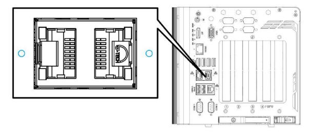
To install and make use to the panel screw hole connection, you must acquire cables with screws shown in the illustration below.
