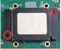
Screw holes for CPU retention bracket
