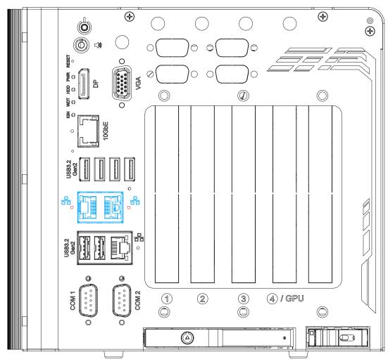
The systems has two 2.5Gb Ethernet ports feature panel screw fix holes (indicated in **red**). Each port has one dedicated PCI Express link for maximum network performance. Please refer to the table below for LED connection statuses.
