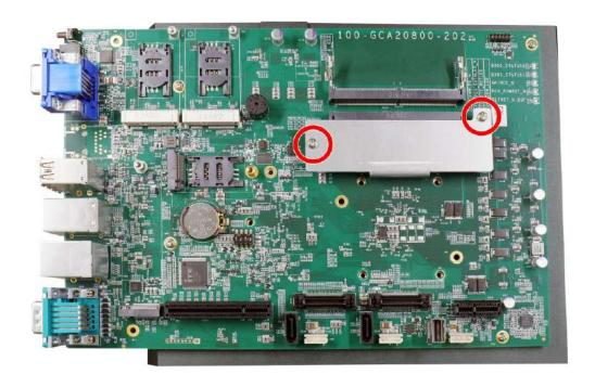
Screws on the memory module's heatsink
