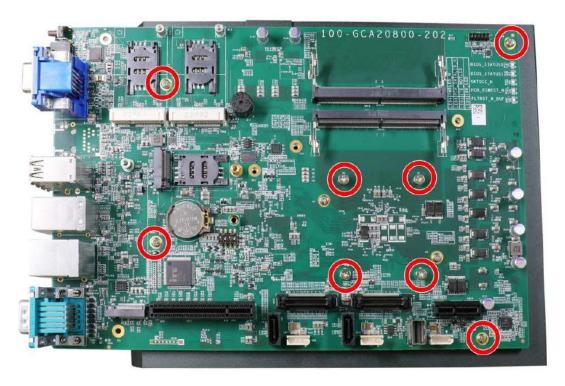
3. Gently separate the motherboard from the heatsink. With a hand on the CPU retention bracket, remove the screws indicated to remove the CPU holder from the CPU.
