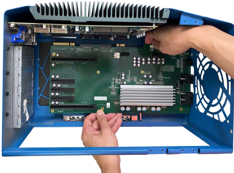
Disengage the daughter-board from the motherboard
