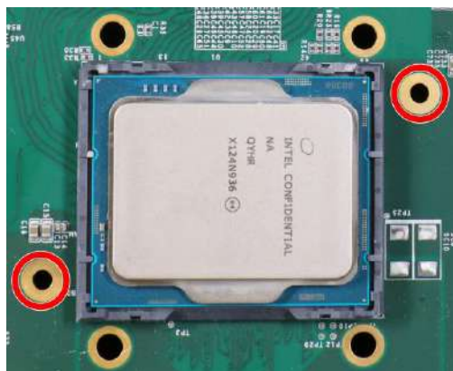
Screw holes for CPU retention bracket
