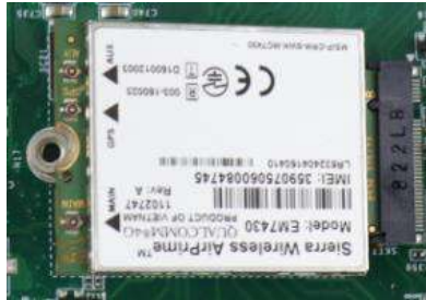
Insert on 45 degree angle
