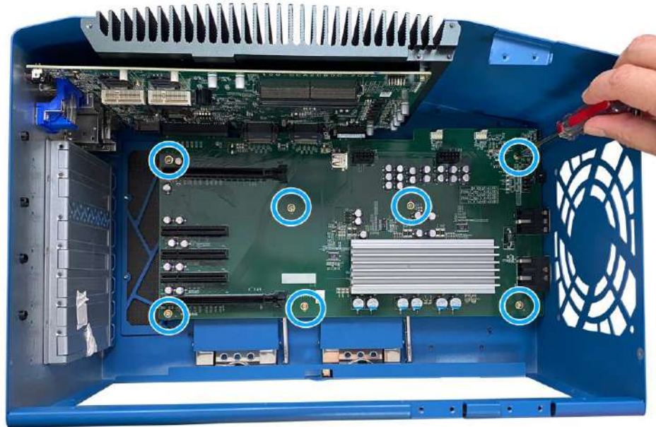
Remove screws securing the daughter-board
