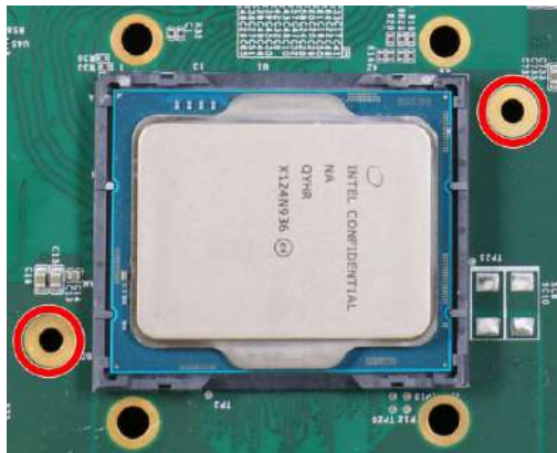
Screw holes for CPU retention bracket
