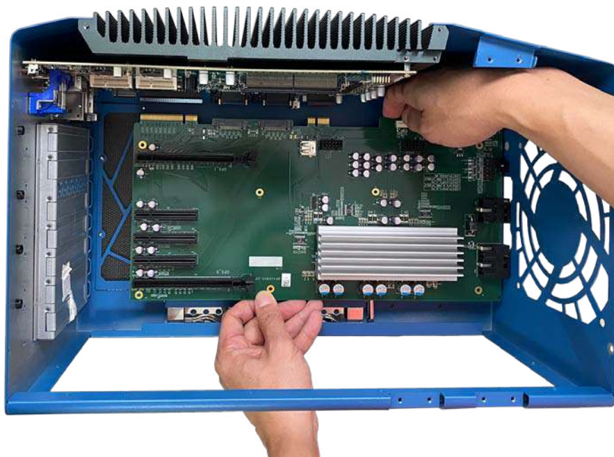
Disengage the daughter-board from the motherboard
