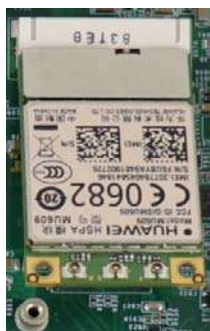
Insert on 45 degree angle
