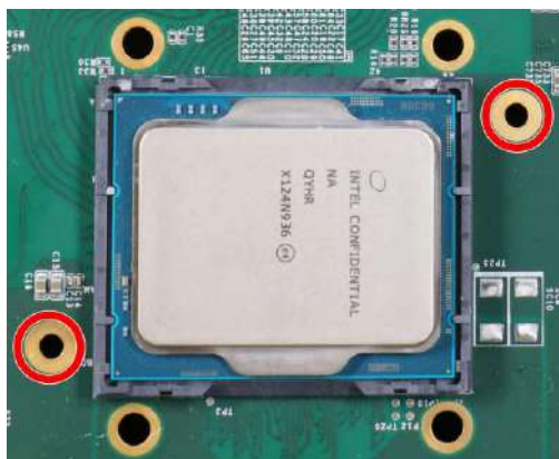
Screw holes for CPU retention bracket
