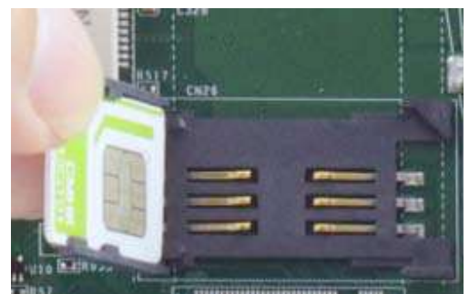
Insert Mini-SIM card with pins facing up
