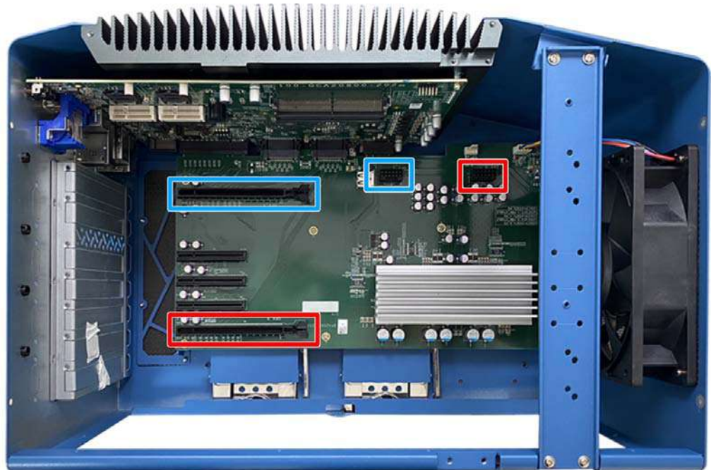
Matching power connectors to PCIe slots
