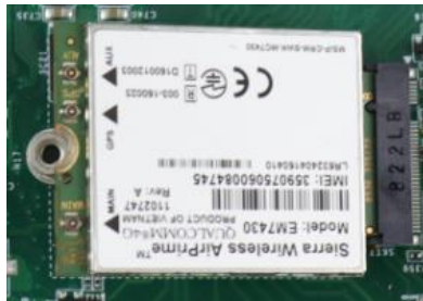
Insert on 45 degree angle
