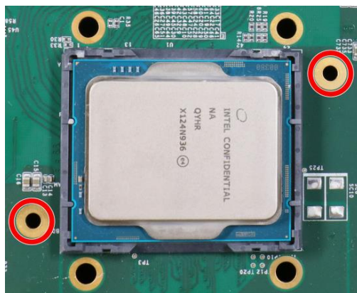
Screw holes for CPU retention bracket
