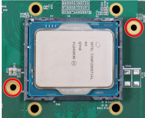
Screw holes for CPU retention bracket
