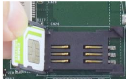
Insert Mini-SIM card with pins facing up
