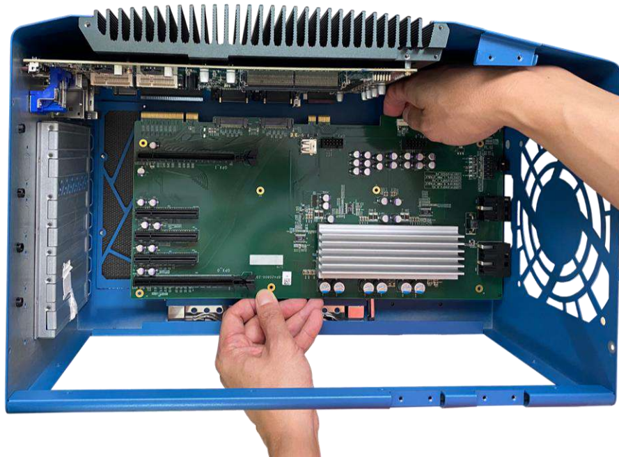
Disengage the daughter-board from the motherboard
