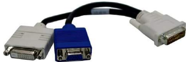
Optional DVI to VGA+DVI Y-cable
