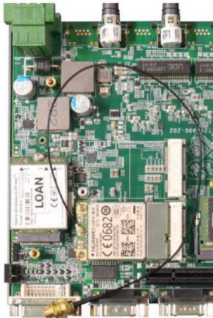
Clip on the IPEZ-to-SMA cable
