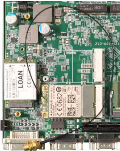
Clip on the IPEZ-to-SMA cable
