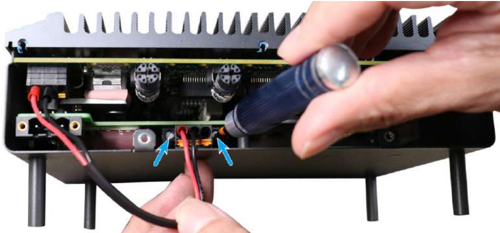
Release screws on the 3-pin connector
