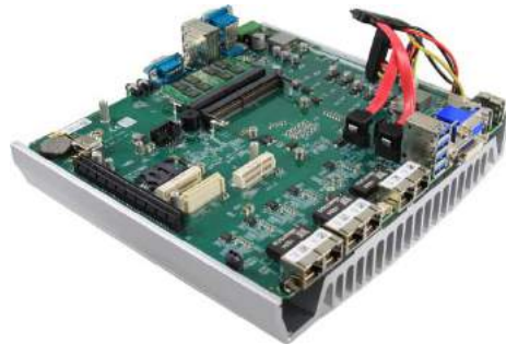
Press down on the outer edge of the memory module
