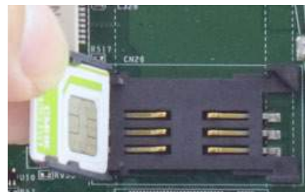
Insert SIM card with pins facing up
