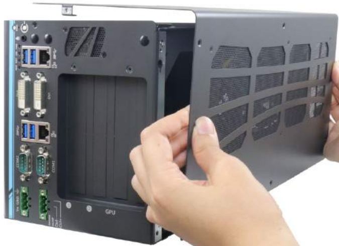
Place side panel onto enclosure
