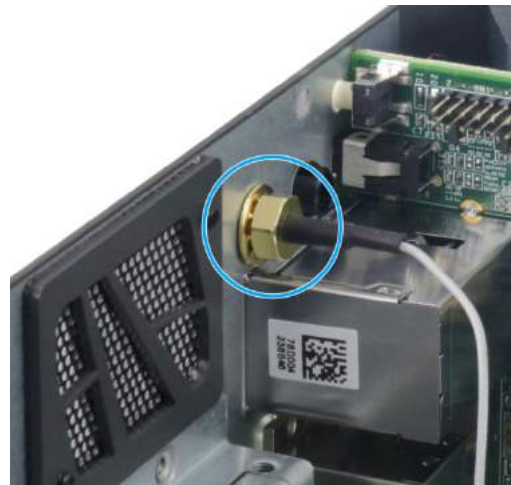
Secure antenna to rear panel
