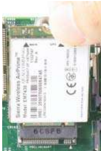
Insert on 45 degree angle
