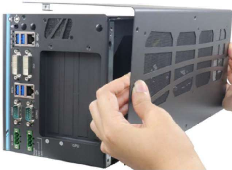
Place side panel onto enclosure
