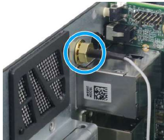
Secure antenna to rear panel
