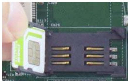
Insert SIM card with pins facing up
