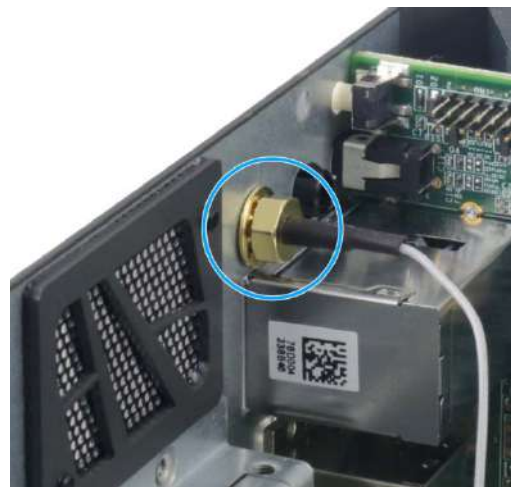
Secure antenna to rear panel
