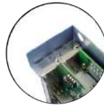
Make sure the card is inserted into the notch and secured with a screw
