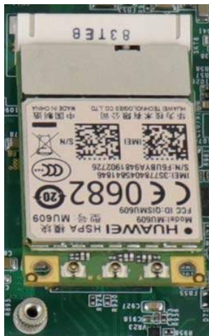
Insert on 45 degree angle
