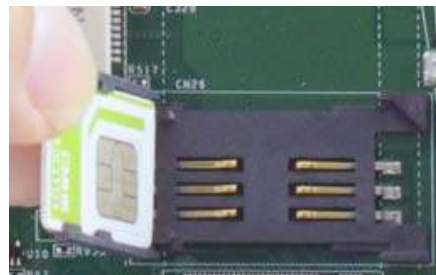
Insert Mini-SIM card with pins facing up
