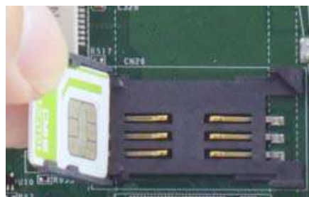
Insert Mini-SIM card with pins facing up
