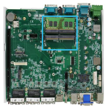
3. To install the memory module, insert gold fingers into the slot at 45-degree angle, push down on the memory module to clip the module into position.
