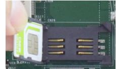
Insert Mini-SIM card with pins facing up
