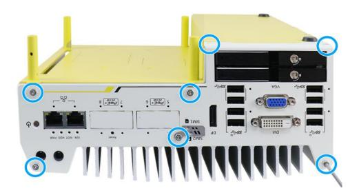
2. Install the front panel and secure screws indicated in **blue**.
