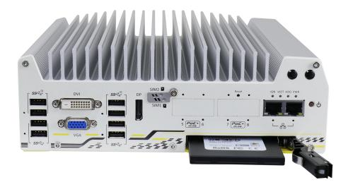
4. Push the lever into the 2.5" slot until it snaps into position. A key is provided (in accessory box) to lock the external slot.
