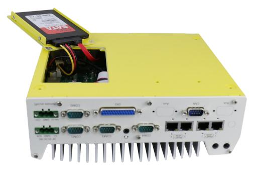
5. Gently put the tray back into the system with the connector side being inserted into the system first and secure the tray with three screws.
