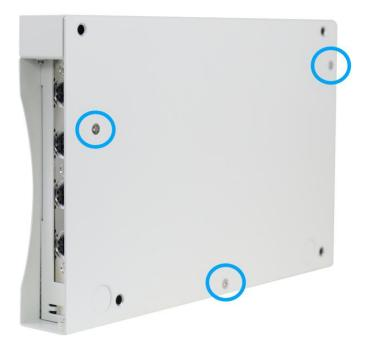
6. Gently lower the Cassette module back onto the system enclosure and secure the module onto the system enclosure by securing the following screws.
