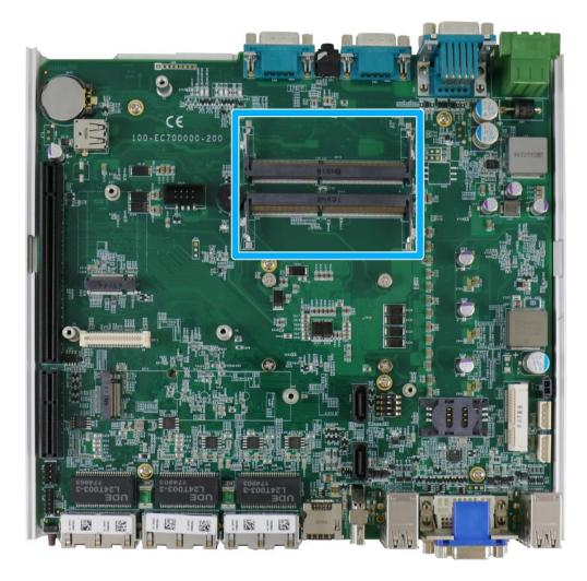
The system motherboard supports two 260-pin SODIMM socket for installing DDR4 memory module up to 64GB. Each slot supports single module DDR4 2666MHz SODIMM up to 32GB capacity.
