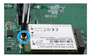
5. Clip on the IPEZ-to-SMA cable to the module and secure the antenna to the front or rear panel. Please refer to the module's manual for clip-on connection.
