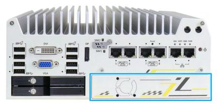
The Cassette module provides a separated compartment to accommodate an add-on card. It compartmentalizes the heat generated and effectively manages thermal conditions of both the system and add-on card(s). The modular design reduces the complexity of installing and replacing add-on card to offer system stability and reliability. To install a PCIe card into the Cassette module, please refer to the following procedure: 1. Turn the system upside-down and remove the four screws.
