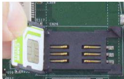
Insert Mini-SIM card with pins facing up
