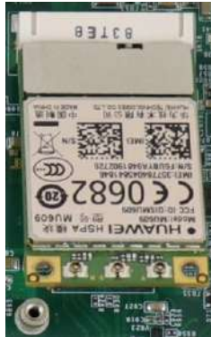
Insert on 45 degree angle
