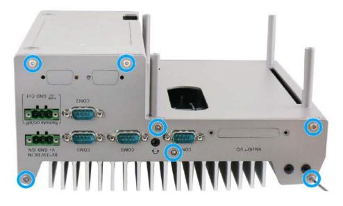
Install rear panel and secure screws
