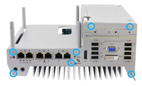
2. Install front/ rear panel and secure screws indicated in blue.
