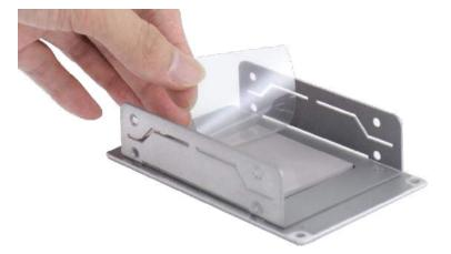
Place the HDD/ SSD (with labels facing up) and match the SATA connector end to the side with two screw holes (indicated in blue), secure the HDD/ SSD with the supplied flathead screws (4 per drive).
