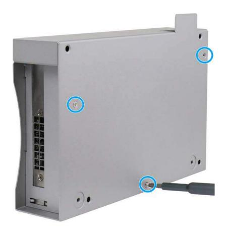
10. Gently lower the Cassette module onto the system, press firmly to ensure the PCIe slot is properly engaged and secure the Cassette module.
