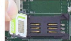
Insert Mini-SIM card with pins facing up
