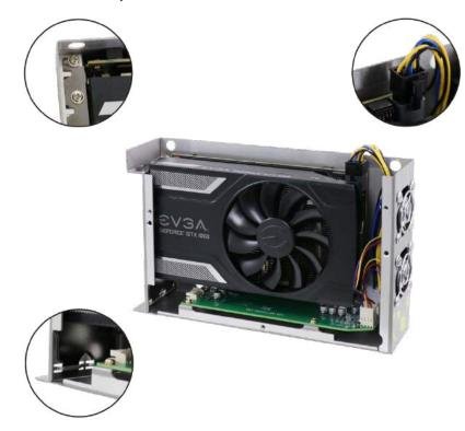
7. If you need to remove the graphics card out of the Cassette module, remove the screws, disconnect the 6-pin connector and flip the white lever outwards to disengage the PCIe slot.
