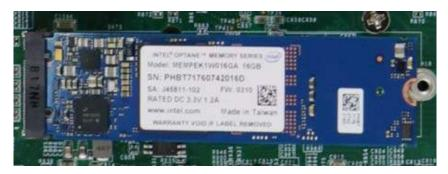
3. Gently press down and secure the module with an M2.5 P-head screw.
