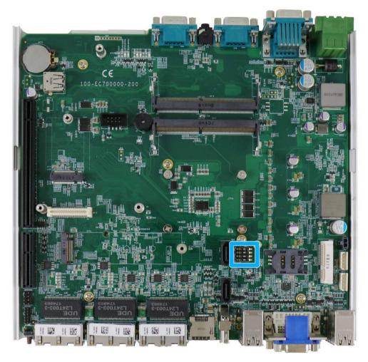
The DIP switch (indicated in **blue**) should be already configured out of the factory. Users need only set the 4th DIP switch to ON for BIOS update and switch back it to the OFF position when BIOS upgrade has completed. The table below shows the system default DIP switch settings for reference purposes.
