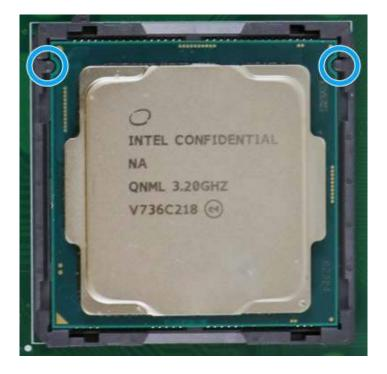
5. Locate the CPU retention bracket from the accessory box. Place the retention bracket on the CPU and hold it in place.
