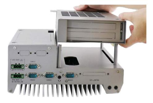
4. Secure the screws indicated to complete the enclosure installation process.
