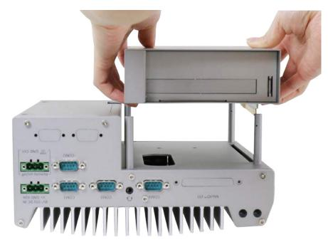
2. Gently wiggle the Cassette module and separate it from the system enclosure.
