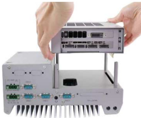
Lower Cassette module onto system
