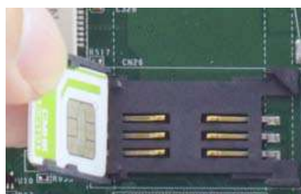
Insert Mini-SIM card with pins facing up
