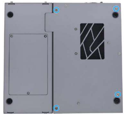
Secure Cassette with screws
