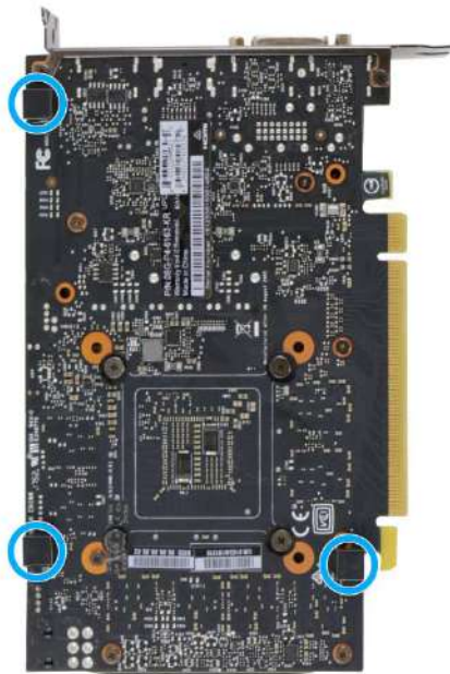
3 rubber stands on back of graphics card
