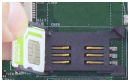
Insert Mini-SIM card with pins facing up
