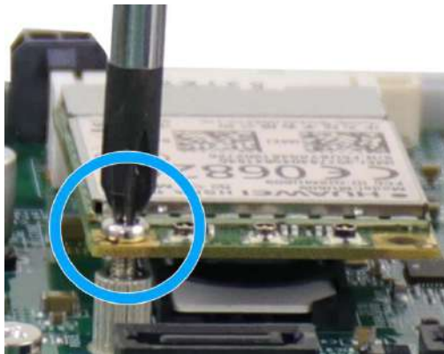
Insert on 45 degree angle Secure the module
